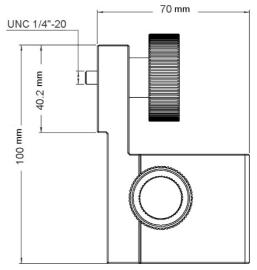
For coarse and fine adjustment of Working Distance and/or Focus of Inspectis Digital Microscopes. Especially advantageous when macro lenses +3, +5 or +10 macro lenses are used.
