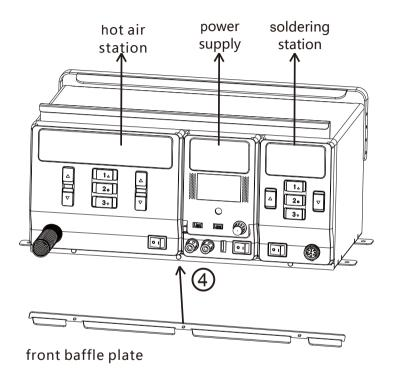
(3) hot air station, power supply, and soldering station inside to fixed cover from left to right.
